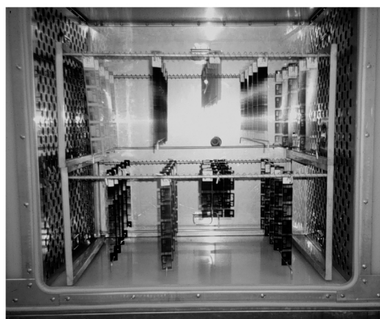
Photographic samples inside a simulated pollutant test chamber at the Image Permanence Institute.
