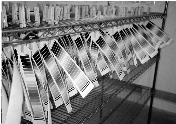
Some of the hundreds of photographic color paper samples used in the University of Rochester/IPI research project on color image stability.
