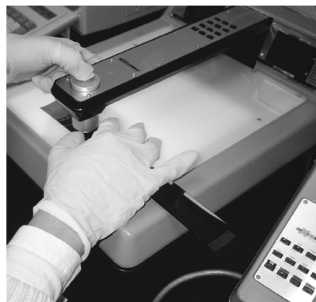
A densitometer was used to measure the fading behavior of color photographs in this research project.
